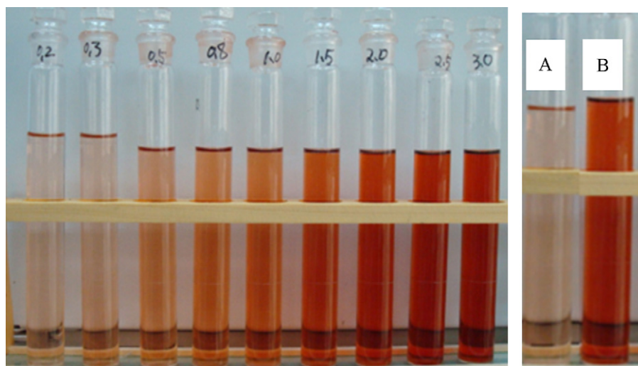
Fig. 3. The standard solution (left) with nine contents of Fe 3+ : 0.2, 0.3, 0.5, 0.8, 1.0, 1.5, 2.0, 2.5 and 3.0 wt.%; Tested samples A and B solution (right).
